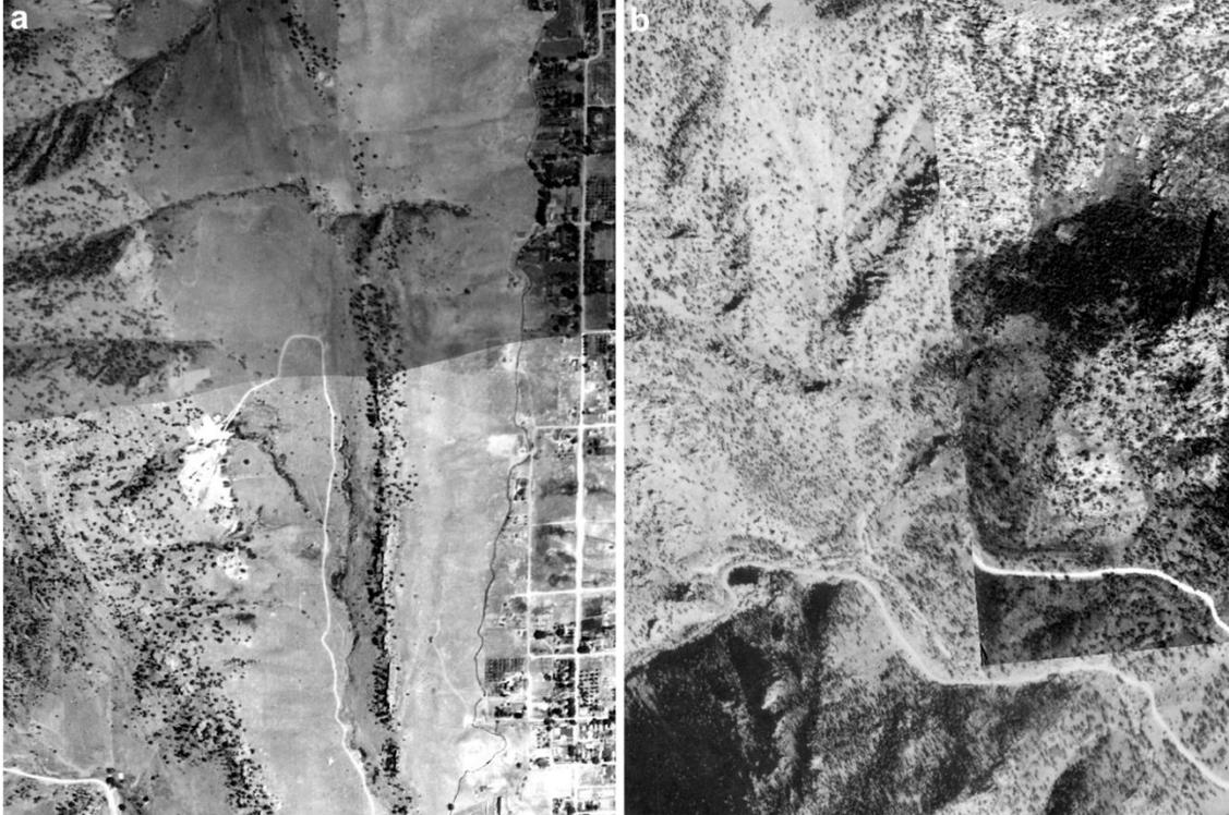
Figure 6: Some of the issues with merging adjacent air photos into a single photo mosaic. (a) Visible tonal differences at scene edges following mosaicking in the eastern flight line, and uncorrected offset between adjacent flight lines (b). Frame (b) will ultimately look like (a), and the full mosaic will then be tonally corrected in Adobe Photoshop CS6. However, image segmentation also corrects for some of these tonal differences in the classification process.
