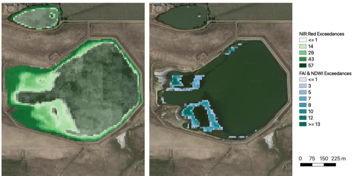
Figure 8. The number of exceedances counted using the NIR:Red threshold (left) and the FAI and NDWI thresholds (right) from April 1 st 2019 through October 31 st 2019 at Lagerman Reservoir. The greater the number of exceedances, the more persistent a probable algal or cyanobacterial bloom may be. Satellite imagery: © 2020 Google, CNES / Airbus, Maxar Technologies, Public Laboratory, U.S. Geological Survey, USDA Farm Service Agency.
