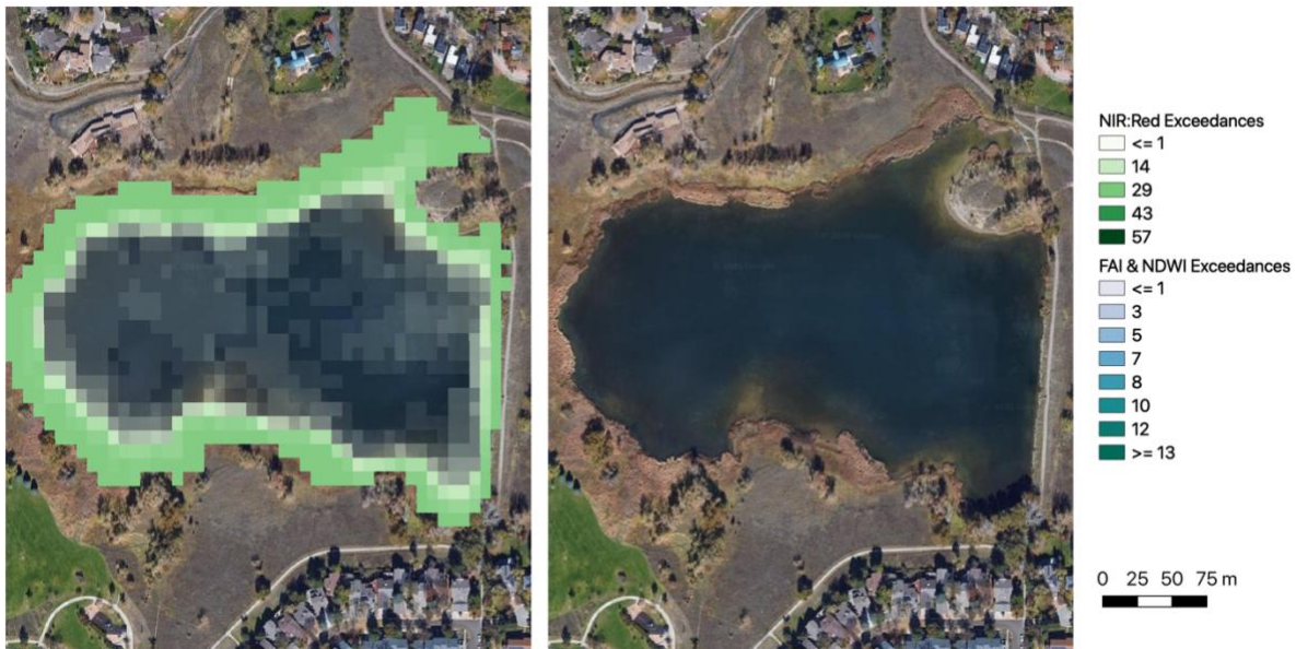
Figure 14. The number of exceedances counted using the NIR:Red threshold (left) and the FAI and NDWI thresholds (right) from April 1 st 2019 through October 31 st 2019 at Wonderland Lake in Boulder. The greater the number of exceedances, the more persistent a probable algal or cyanobacterial bloom may be. Satellite imagery: © 2020 Google, CNES / Airbus, Maxar Technologies, Public Laboratory, U.S. Geological Survey, USDA Farm Service Agency.
