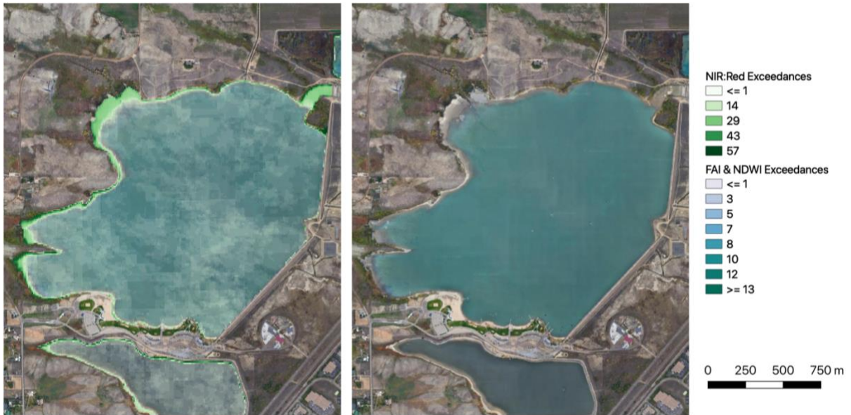
Figure 7. The number of exceedances counted using the NIR:Red threshold (left) and the FAI and NDWI thresholds (right) from April 1 st 2019 through October 31 st 2019 at Boulder Reservoir. The greater the number of exceedances, the more persistent a probable algal or cyanobacterial bloom may be. Satellite imagery: © 2020 Google, CNES / Airbus, Maxar Technologies, Public Laboratory, U.S. Geological Survey, USDA Farm Service Agency.
